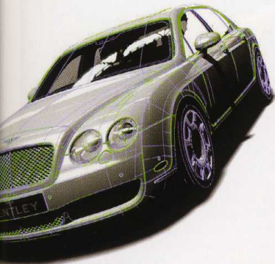
The Bentley Continental Flying Spur inside ICEM Surf with the patch structure and menus turned on. This level of visual realism is real time and persistent, which means that the designer can model and work at this level all the time without resorting to stand-alone visualisation tools
